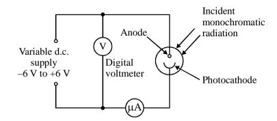
The incident radiation has a wavelength of 215 mm. The metal surface of the photocathode has a work function of 2.26eV.
