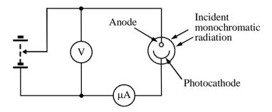
As the reverse potential difference between the anode and cathode is increased, the current measured by the microammeter decreases. When the potential difference reaches a value  $V_s$ , called the stopping potential, the current is zero.
